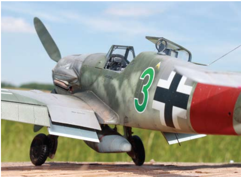
Dropped flaps, a new tank and a new tail and horizontal stabilizers are among the aftermarket additions to this Bf 109G-14/AS.
